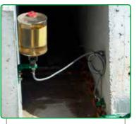
02.900.000 Automatic greasing system for turning chain incl. oil 5 litres
